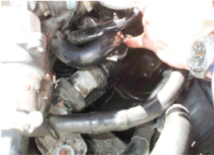
Old ARP with pinky in coolant hose. Electrical plug is disconnected.
