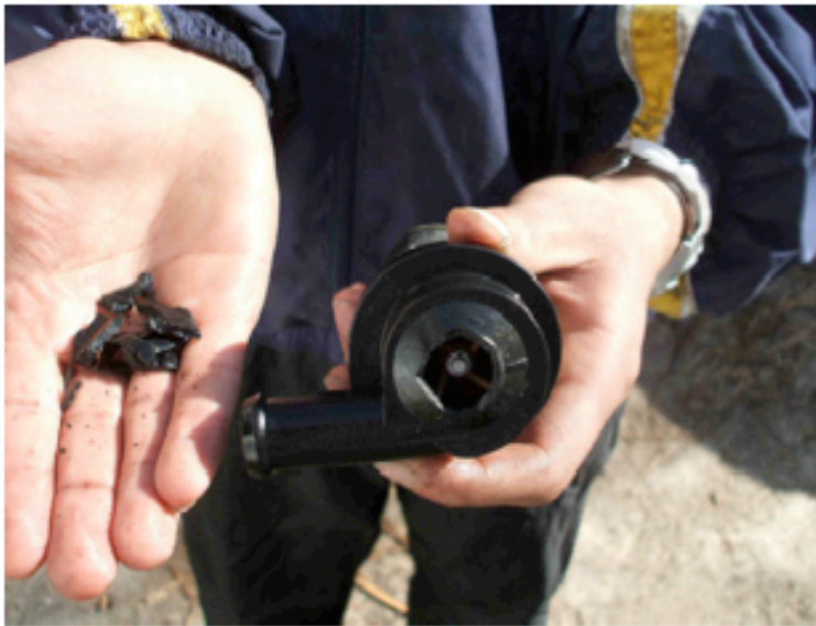
Old ARP with plastic bits that broke. Check out that impeller.
