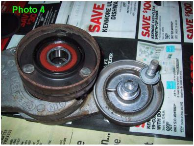
5. The roller is made of 3 pieces – a ring that takes the dust cap and two roller halves (see Photo 6). The entire assembly is riveted together. Each half is flanged over the bearing, so the bearing cannot be pressed out –
