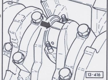
Compare width of Plastigage strip with measuring scale.
