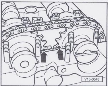
When installing bearing caps, recesses on corners of caps must point toward intake side of cylinder head (arrow).
