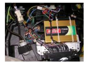
The aluminium cover was deliberately left off the chassis to aid cooling of the MOTEC ECU. The 3 bar sensor is the black blob atop the ECU. It can be replaced by a 5 bar sensor by the brave (or foolish) who seek such levels of boost. Next, the oxygen sensor was replaced by a wide-band OXS that works with the MOTEC (see picture).
