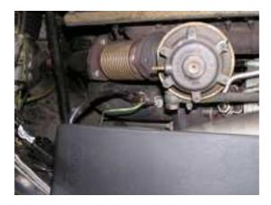
(The green wire goes to an exhaust gas temperature probe, used in earlier testing, and since removed). Finally, the MAF was removed, and replaced with a tube of the same external shape that Neil turned from a solid block of industrial strength Nylon (see picture).
