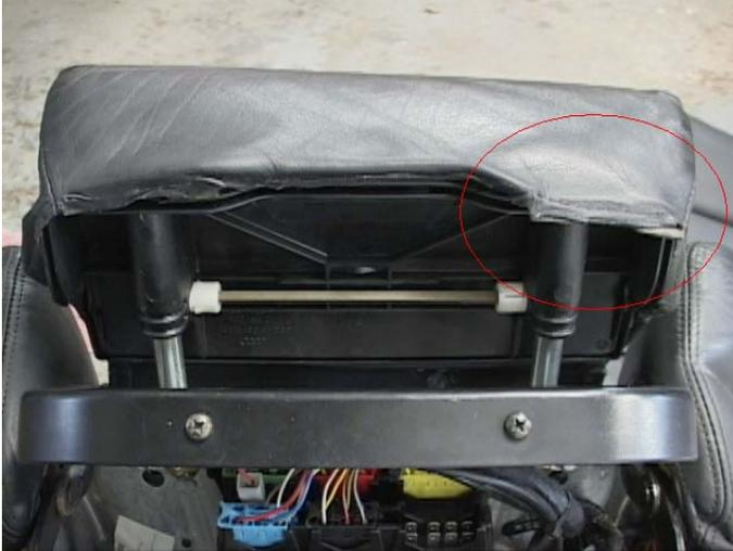
Now look at the rear of the base. Remove the two plastic sleeves from the posts where the torx bolts used to live. Loosen the 17 mm bolt that attaches the seat belt receptacle to the base and remove the plastic guard that is also attached to the torx bolt post. Slide the heavy cloth material and the leather off the post.
