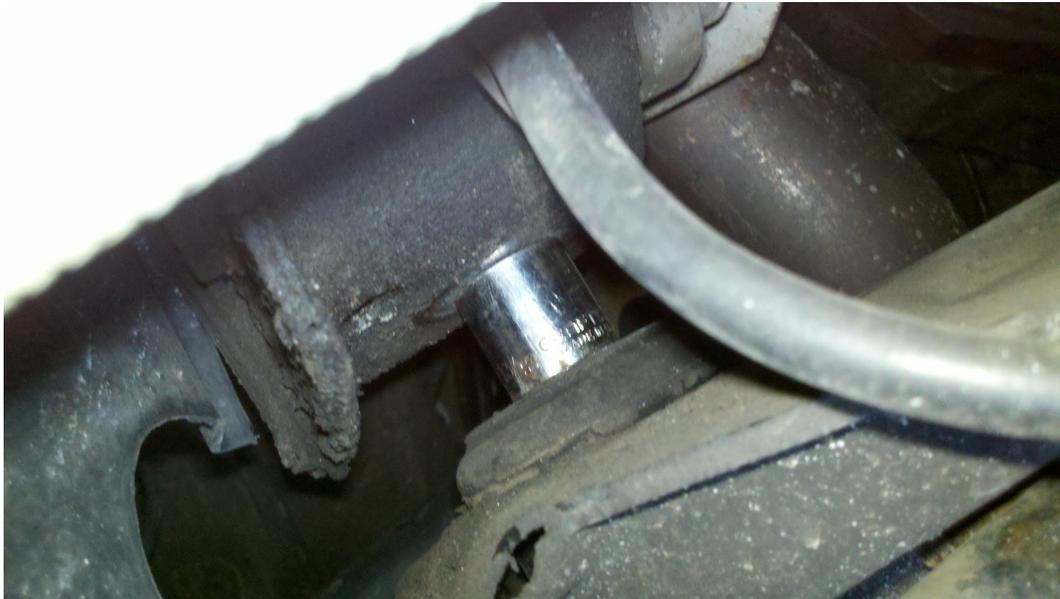
Using the floor jack, jack the subframe up. The socket will push the old subframe bushing out as it draws closer and closer until it pops completely out. Clean up any metal shavings you may have and other debris. Make sure all surfaces the bushing will be in contact with are completely clean.
