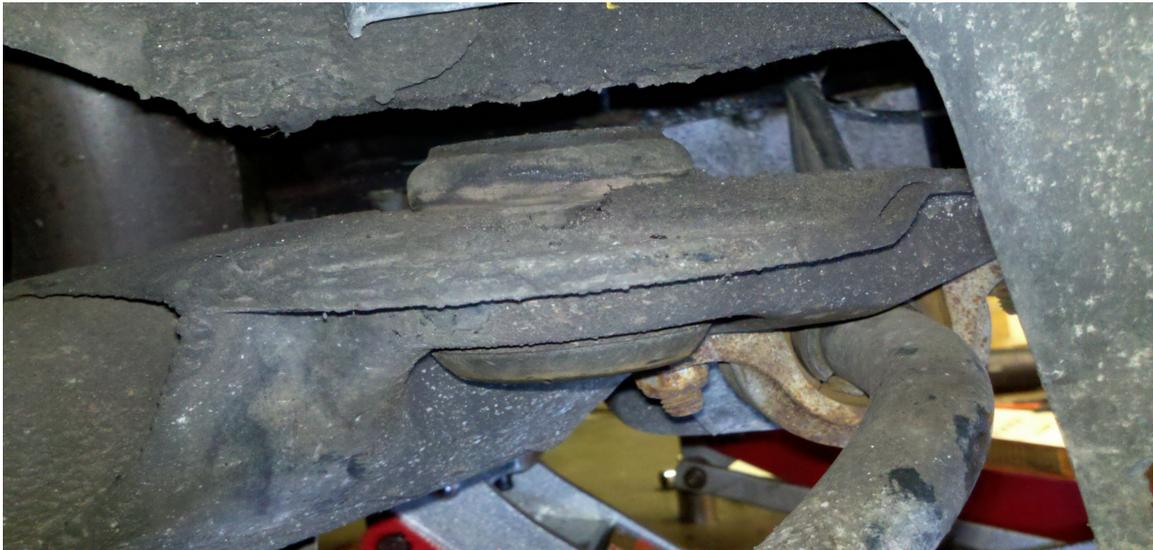
I used a sawzall with a metal cutting blade to make a horizontal cut. Looking at photo #2 above, imagine the blade placed flush against the top of the subframe on the left hand side of the bushing, cutting towards the front of the car (this is the passenger side bushing). With the top of the bushing now cut off, I placed a socket in between the now cut bushing and chassis above it. See the following photo:
