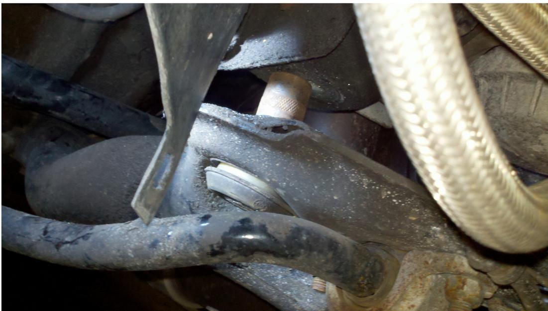
Position your lubricated bushing for installation. I placed a large socket on top of the floor jack and positioned the socket against the bottom of the new bushing. Slowly jack upwards. The socket above the subframe should keep it from moving up. This allows the larger socket underneath to push the bushing into place. Once the bushing is seated, remove the sockets and jack the subframe back up into place and reinstall both bolts. That should do it!
