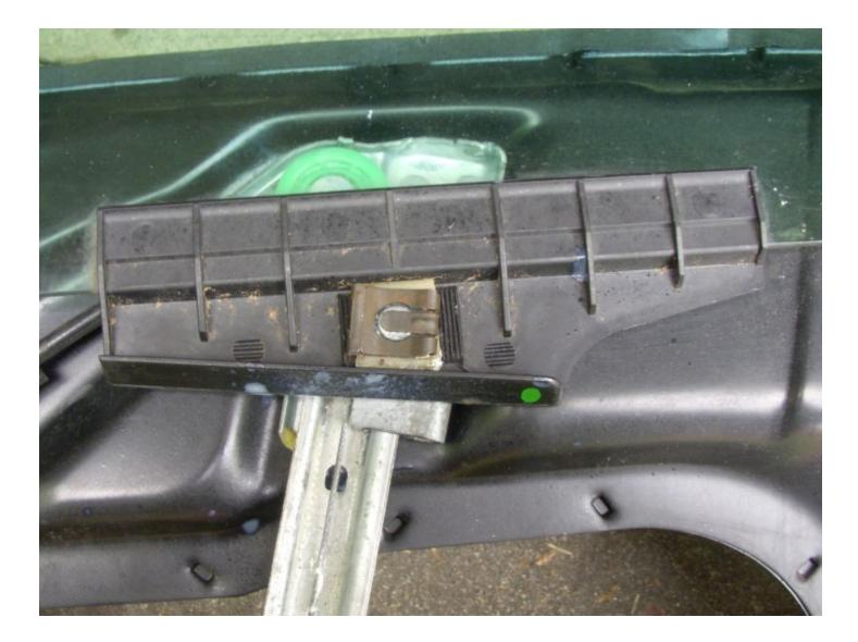
The glass has some flex and can be lifted up and over the pin that square white positioning washer is around and the clip is over (once both are removed).
