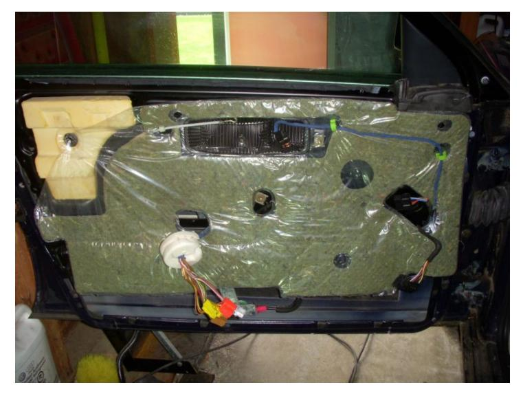
Note the location of the wiring including the green clips holding the blue wiring bundle to the door lock switch. The window switch wiring is with the big white foam plug on the middle left. The seat/mirror memory switch wiring and the door speaker wiring in on the lower right.
