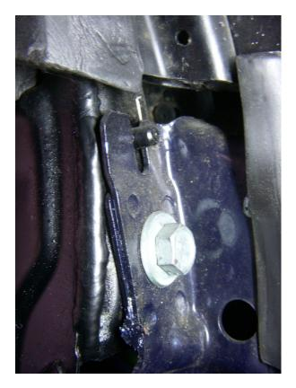
Here is a photo of the lower bolt with a "peak-a-boo" view of the aluminum "U" shim (bottom, middle-right) and one of the electrical harness connectors that have to come off the window cassette before it can be removed from the car.
