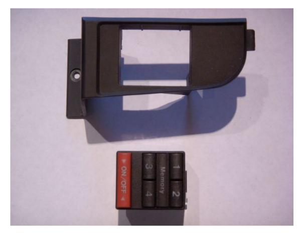
Take the switch and install it onto the harness plug in the door panel:
