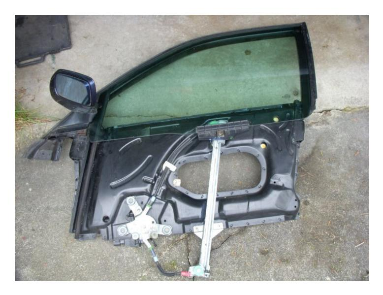
Yup. The window cassette is also the upper part of the door as well as holding the window and the window regulator and the mirror. It must be made of aluminum because even with the glass, it isn't that heavy. This photo was taken after I got out the old glass (a very tiny piece connected to the black plastic connector piece) and cleaned things up and put in the new glass. But this is skipping ahead. First we need to get the window cassette out of the car.
