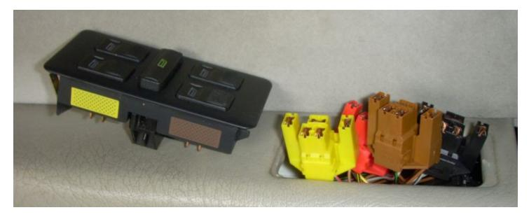
So assuming you followed either Jimmy's or Marv's panel removal DIYs and you are ready to remove the panel, there are a couple of extra driver's door issues. This first is to pull the window switch wiring out of the back of the door panel, removing the big white foam sealing plug as you do so:
