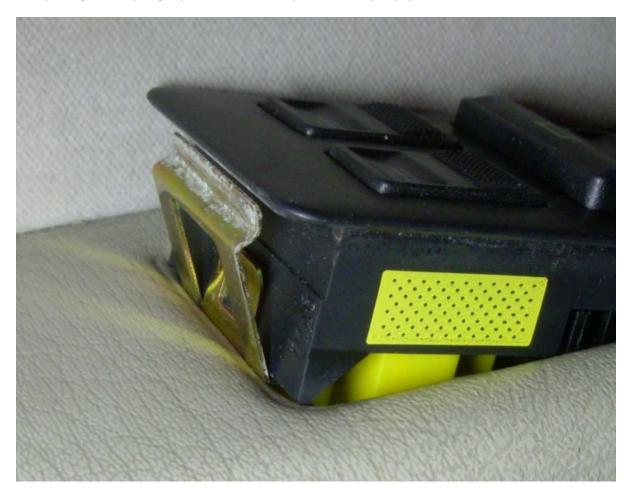
Before you go ahead, if your glass isn't broken, turn the ignition to RUN and use the window switch to run the glass all the way into the door. To remove the switch panel, you need to use a putty knife to get under the rear edge of the window switch panel and onto the upper edge of the spring clip. Us a 1.25" (31 mm) putty knife or stiff(er) equivalent. Get it under the lip of the switch panel. Angle it down to catch the top of the metal spring clip, then push in and pry up:
