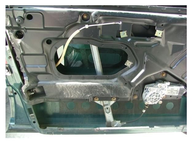
For those that notice details, you might have noticed that Marv's 92 UrS4 window regulator is bolted to the window cassette frame, whereas the regulator for my 98 C4 Avant is riveted into the window cassette frame. The change occurred sometime with the UrS6s. Doesn't matter - unless you are also replacing the window regulator.
