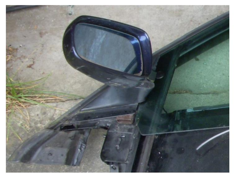
Once you have the window cassette free, place it down gently somewhere safe where you can work on it. I put in the back of the avant with the hatch open. A big table on a blanket would work too. Now go back to the door.
