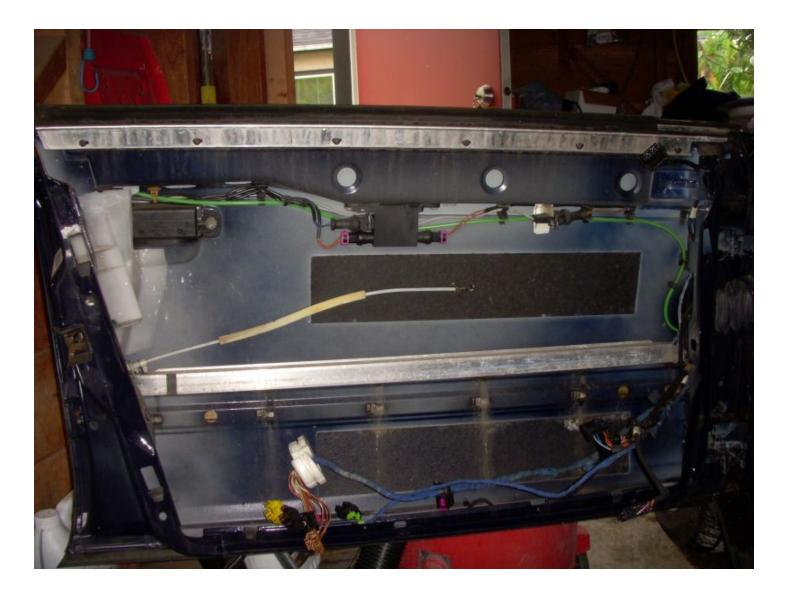
While you have the vacuum out, vacuum all the broken glass and debris out of the window cassette, paying close attention to the tracks in which the window guides run up and down.
