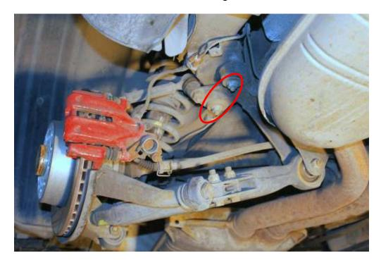
4) Position the sway bar mounting plate as shown, and reinstall the subframe nuts. The two smaller threaded holes in the sway bar bracket should be offset to the passenger side.
