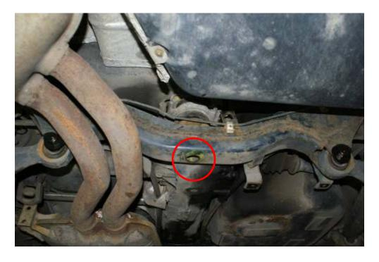
3) Remove the two driver's side subframe nuts using a 17 mm socket.
