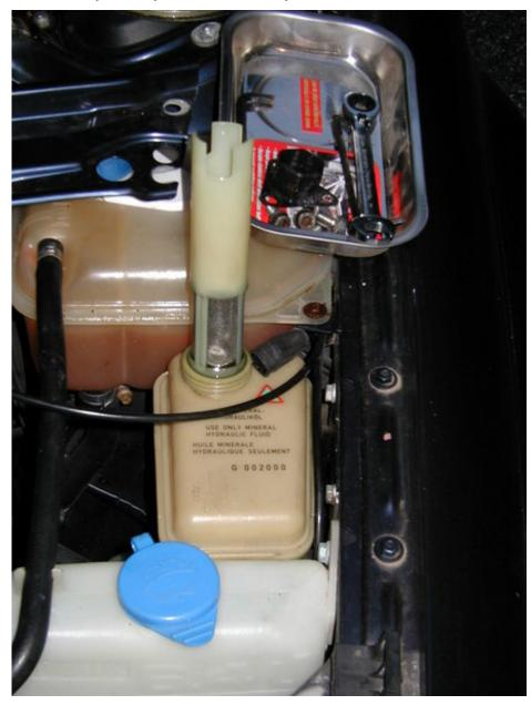
If possible, pinch off the supply hose as shown, and then remove.
