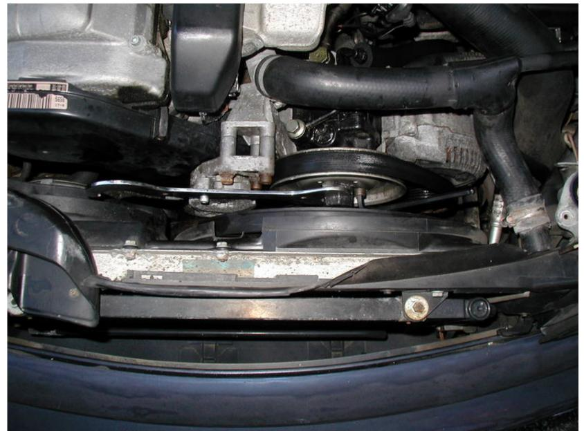
Once the pulley is removed, it's time to drain the hydraulic reservoir. Always remove the wire for the fluid level sensor before trying to unscrew and remove the cap.
