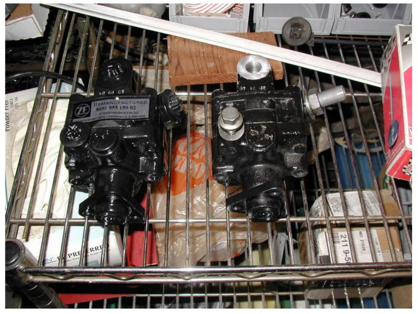
Once the inlet tube is swapped, reinstall the pump. Prime both halves of the pump with the turkey baster, then reattach the supply hose and turn pump until fluid comes out both ports. If necessary, use your Mitvac or equivalent to help prime the HP side- you absolutely want to see fluid coming out of both ports before reconnecting the high pressure hoses, since these pumps do not last long if they're run dry.
