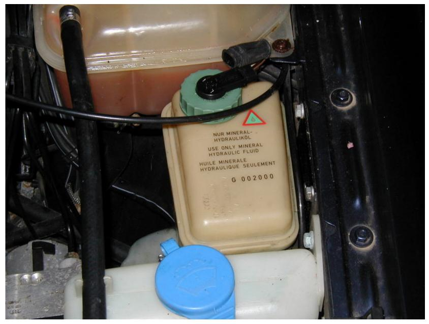
Once the cap is off, remove the filter. It just slides up and out. When the filter is out, use a turkey baster to remove as much fluid as possible. If the reservoir still has the factory crush clamps on the supply and return lines, take the opportunity to pull the reservoir and replace both with screw clamps.
