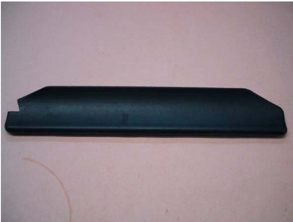
Photo 5 Foil topside – note clearance notch cut out of right side.
