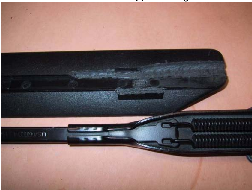
Photo 7 Clearance groove cut in foil
