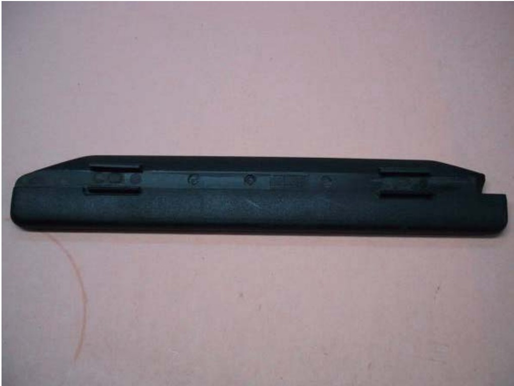
Photo 4 Underside of foil – note arm mounting surface
