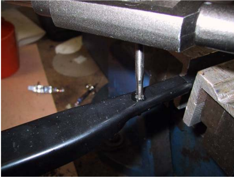
Photo 8 Drill and tap wiper arm
