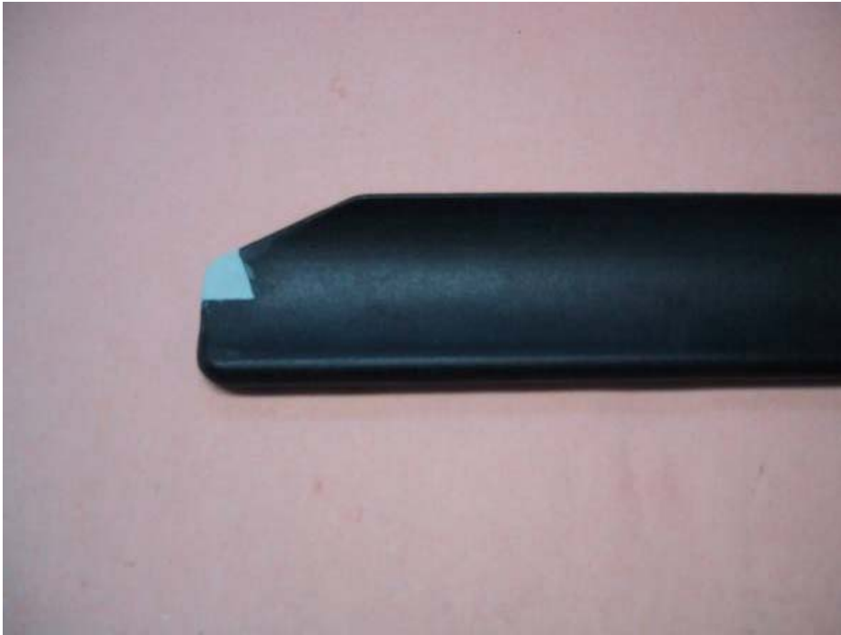
Photo 6 Clearance notch filled and faired.
