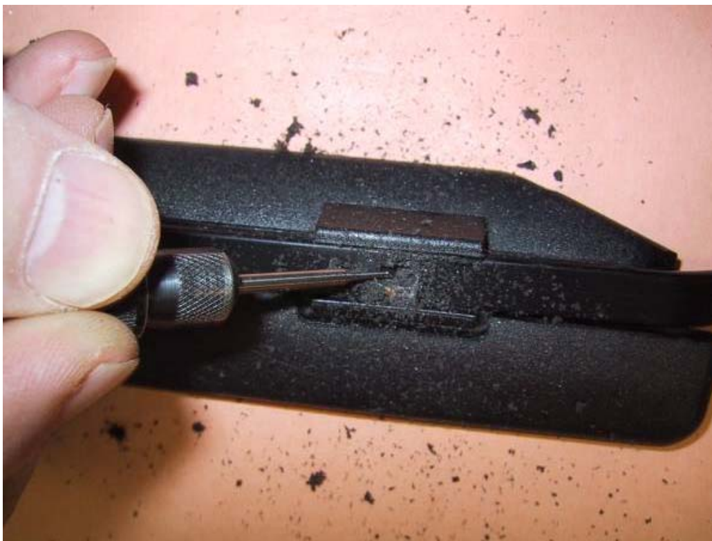
Photo 3 Cut out plastic retaining pins
