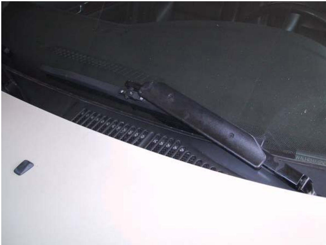
Photo 11 Completed WiperWing assembly
