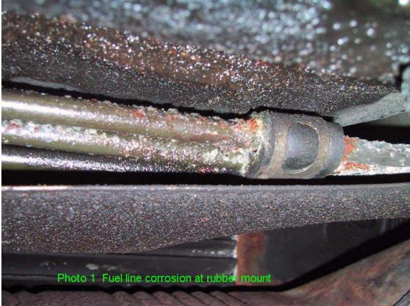
1. Photo 1 shows what a corroding line looks like. This was the most corroded area on my car and the spot the line eventually failed.
