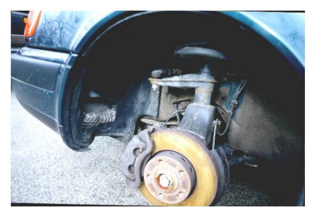
After some minor trimming, six No. 8 panhead self-tapping screws (as short as you can get them, e.g. 0.5" or less) were used (3 per side) to fasten the S4tt louvers into the UrS4 liner. Pop-rivets would have worked fine too. The UrS4/Frankenliner was then reinstalled into the wheel well. End result,: Looks Good!! (Does it work? Time will tell).
