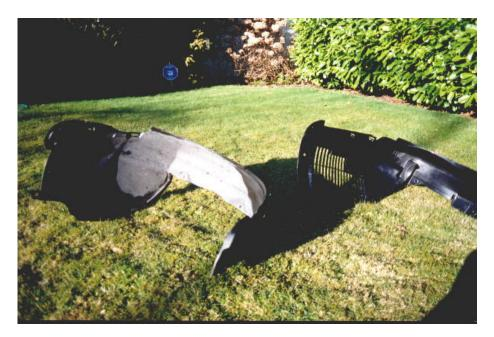
The UrS4 liner comes out easily (once you see the single black screw on the upper wheel well lip). Once the liner is out you can see how poorly the airflow through the intercooler really is. There is no clear way for the hot air to get out of that area. I bet that whole area is slightly pressurized and there is very little flow of cool air through the intercooler.
