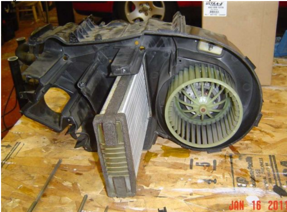
Photos courtesy of Mark A. (Thefeek) This photo, taken during Sean D's (quattro20V's) heater core R&R, shows the old heater core (with cracked nipples) and the sealant that needs to be cut away in order to be able pull the heater core out of the back of the left side of the heater box:
