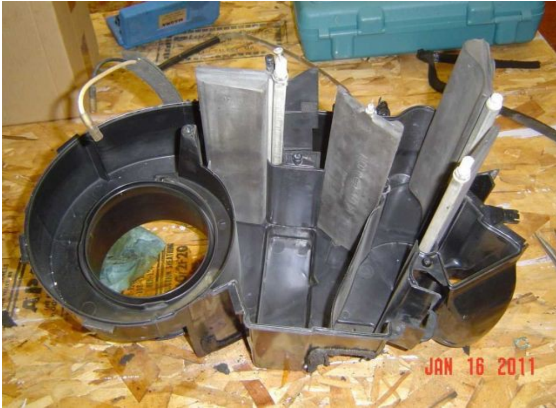
Here is the left side of the disassembled heater box showing the heater core and the blower (Note: The box in the back ground has the PN 4A0959101A = new blower fan on it)
