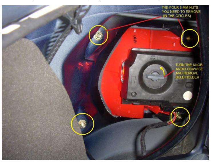
Note: That if you want, you can remove the lamp holder earlier than waiting for all four nuts to be off. Removing the lamp holder might make it easier to access the lower inner nut. Note the black bracket in the lower right corner of this photo:
