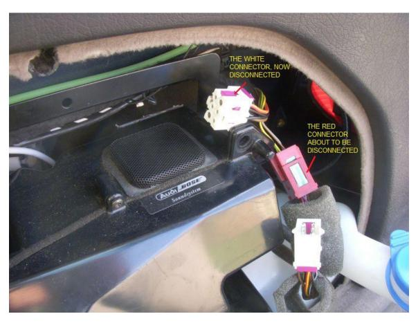
With the electrical connections to the BOSE sub disconnected, pull/wiggle the the sub itself out. IF the loosened bracket is still causing you grief, unclip the wiring harness from the bracket (be gentle with the wire clips, you can re-use them if you don't damage them – wiggle one side of the "^" out and then the other).
