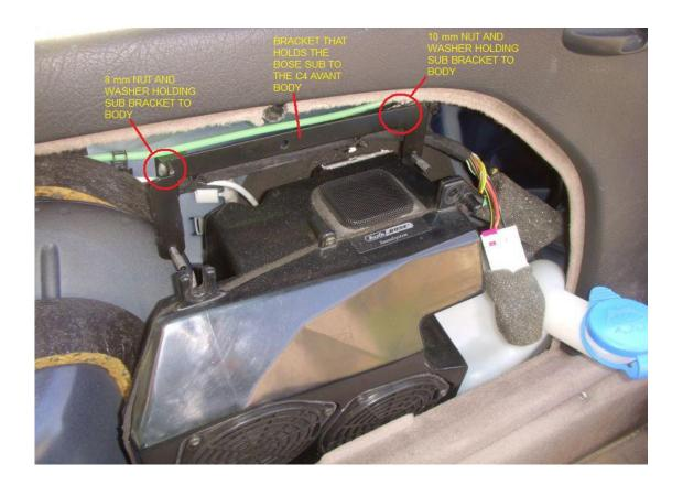
Once the bracket is either out or at least loose, you will be able pull the BOSE Sub out further. However, before you remove the entire sub, you will have to disconnect the red and white connectors that are hiding in their little grey foam sleeves:
