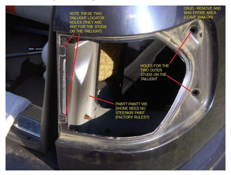
Note the two locator tabs and holes on the inner side (these will be important in a minute). The outer two holes are much larger and are for the outer two studs on the taillight.
