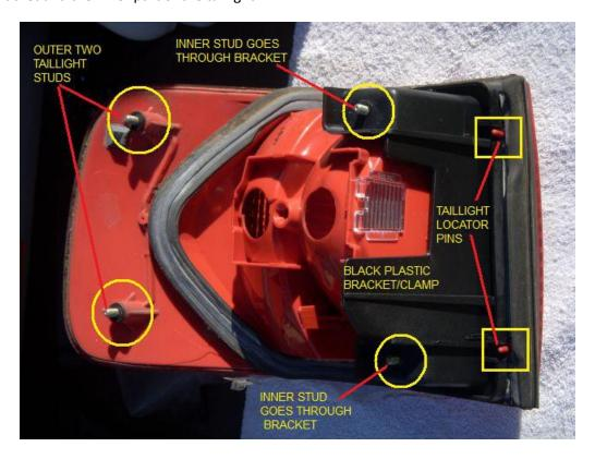
This view shows the bracket/clamp separate from the taillight. Note the "AVANT" branded into the taillight:
