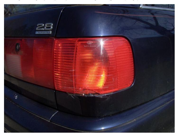
The rear outer taillights are different for the C4 sedans and the C4 avants due to slight curvature differences. Avant outers have "AVANT" branded into the plastic (a photo of this shows up later in this DIY).
