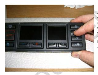
Turn the complete control panel assembly over and test press each button. You should feel that familiar tactile "snap" feedback from each of them. If any button feels "soft" or different than you recall, then remove the circuit board and make sure that the rubber switch pads are all fully seated against the board. Verify that all of the switch pad rivets are fully seated and locked into the board.
