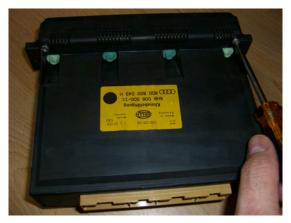
Remove the three Phillips head screws from holding the front control panel to the controller housing. In this photo two screws can be seen at the top. The 3<sup>rd</sup> is on the bottom side. If you do not have the four turquoise lamp holders as seen in this photo, your controller is LED backlit. Rebuild is the same, but you will not need the lamps provided in this kit. If your controller is an early version with a white enclosure, please go to the appendix for updated information.
