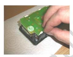
Now do the same on the side with the remaining two tabs; until all tabs of the circuit board are free.
