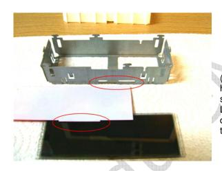
The LCD panel (black) and its color filter (white) removed from the LCD cage. Note how the tab on the color filter fits into the large slot on the LCD cage. If the color filter or the LCD cage require cleaning; do so using only detergent and water. Solvents may damage the paint on the color filter.
