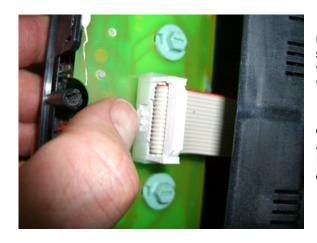
Gently pry outwards on the socket's retaining tab with your thumbnail or flathead screwdriver as shown. Be careful not to pry too much or it may break. Then at the same time pull apart the connector from the socket.
