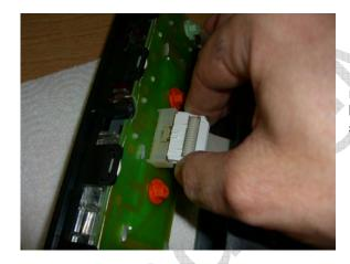
Insert the ribbon connector back into its mating socket on the control panel. There will be an audible click once the connector is fully seated.
