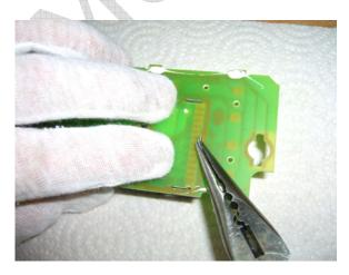
Gently apply downward pressure on the printed circuit board so that the retaining tab can be twisted locking the assembly together.
