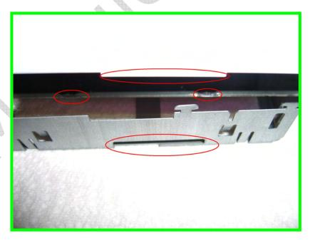
Note that the two LCD fill holes and the tab on the color filter are all oriented the same as the large slot on the LCD cage.
