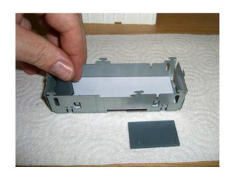
LCD unit with both zebra strips removed. LED backlit displays will have shorter zebra strips
