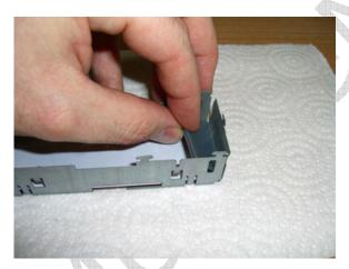
Now remove the right side "zebra strip". The Zebra strip is made from rows of conductive and insulating channels that transfer electrons from the gold pads on the circuit board to the contacts on the LCD glass. The striped pattern is where this connector gets its name. Gently push the zebra connector to the side to release from the LCD and lift it away.
