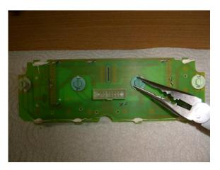
This is the board with the lamps removed. Now is the time to begin disassembly of the LCD itself! The LCD is contained within a steel cage attached to the circuit board by 8 twist lock tabs. Untwist the tabs using your needle nose pliers so the tabs will pass through the slots in the circuit board.
