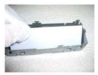
With the color filter stacked on top of the LCD and oriented as instructed, insert them into the LCD cage. Make sure that the tab on the color filter fits into the slot on the LCD cage. Then gently press the filter and LCD flat into the cage. Do not force as they should almost drop into place. If the LCD panel will not sit flat, make sure that the tab of the filter is fitting through the slot on the LCD cage.
