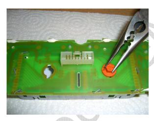
Insert the backlight lamps. These were the two orange or teal base lamps designed to illuminate the LCD panel. These lamps occupy the two inner holes on the PCB directly behind the LCD unit. Insert and then twist ¼ turn clockwise with pliers to lock into place. Repeat with the new green base lamps offered in the kit and fit to the two outermost holes on the circuit board.
