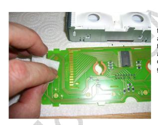
Set the LCD unit aside. Open one of the two alcohol swab pads and use it to wipe down all metallic gold pads on the circuit board. In this photo you can see six gold switch pads and one of the two vertical rows of gold LCD contacts. After cleaning, avoid touching the gold surfaces with your fingers.
