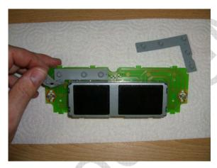
Remove the two silicone button pads from the circuit board. They are simply held in place with integral rubber "rivets" molded into the silicone pads themselves. Simply lift them off the board. Set the silicone pads aside for later.
