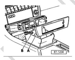
Gently pry wood trim fascia panel (A) from center console using a flat edge tool. A flathead screwdriver with an overlay of electrical tape will prevent any marring of surfaces.
