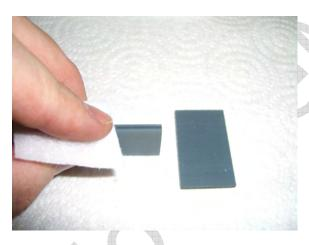
Clean both zebra strips with the second alcohol swab. Wipe down all sides of the zebra strip handling it by the large flat sides paying particular attention to cleaning the edges. Do not allow your fingers to touch the edges after cleaning. If you do by accident touch the edges, just wipe that area again with the swab.
