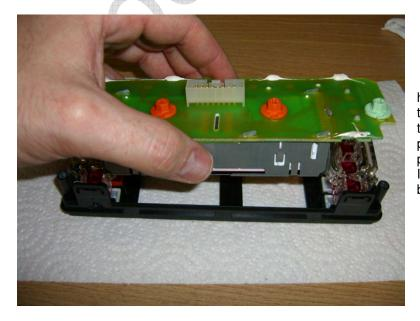
With the control panel housing facing down, lift off the printed circuit board with the LCD display. Set the plastic face panel in a safe place keeping it face down. If you turn it over, all the buttons will spill out.
