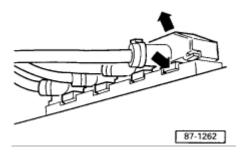
Remove all four electrical connectors by simply pushing the tab in with your thumb and pulling the connector away from its socket. All four connectors are mechanically different to prevent mismatch upon assembly.
