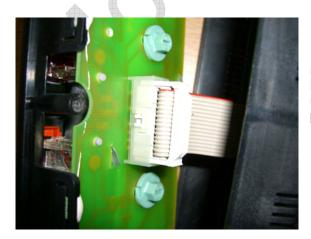
A close up view of the LCD controller board ribbon connector. Note the small retaining latch preventing the connector from being unplugged. LED backlit boards have a lower profile blue connector instead of the white.
