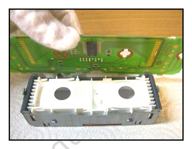
The LCD unit is now complete and ready for assembly with the printed circuit board. The tabs are spaced in such a manner that the board only fits one way – the correct way!
