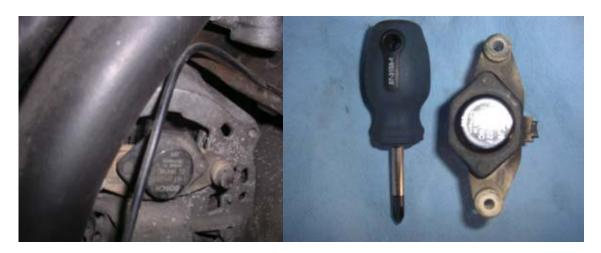
Voltage Regulator removed from Alternator
