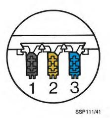
1 = Voltage supply2 = Fast data transfer3 = Flash code
