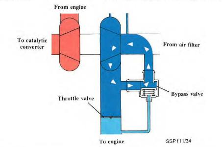
The idle speed is controlled by ignition timing and The idle stabilizer is a single winding rotary-type. an idle stabilizer. The ignition timing is used to When current is supplied to the valve, the rotary quickly adjust the idle speed during load changes. valve will rotate against spring pressure to the desired opening. The opening is determined by the The idle stabilizer is used to maintain the corrected air volume. Motronic control unit.
