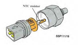
The multi-function temperature sensor is located in the coolant flange on the cylinder head. This sensor has several functions:
