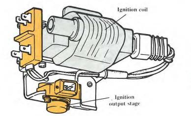
An ignition coil with a separate power stage is used with the Motronic system. The power stage is a Darlington-type of transistor which switches the primary current for the ignition coil on and off.
