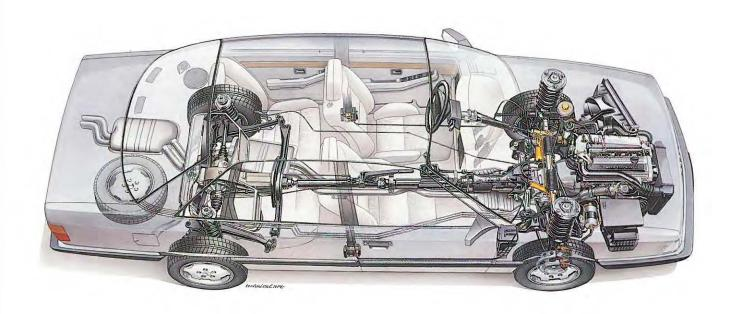
**Technical Data** Type: 5-cylinder in-line turbocharged engine with 4 valves per cylinder Displacement: 2226 cc 86.4 mm Stroke: Bore: 81.0 mm Compression: 9.3:1 Horsepower: 217 @ 5,700 rpm Maximum torque: ·228 @ 1,950 rpm Engine Management System: Motronic
