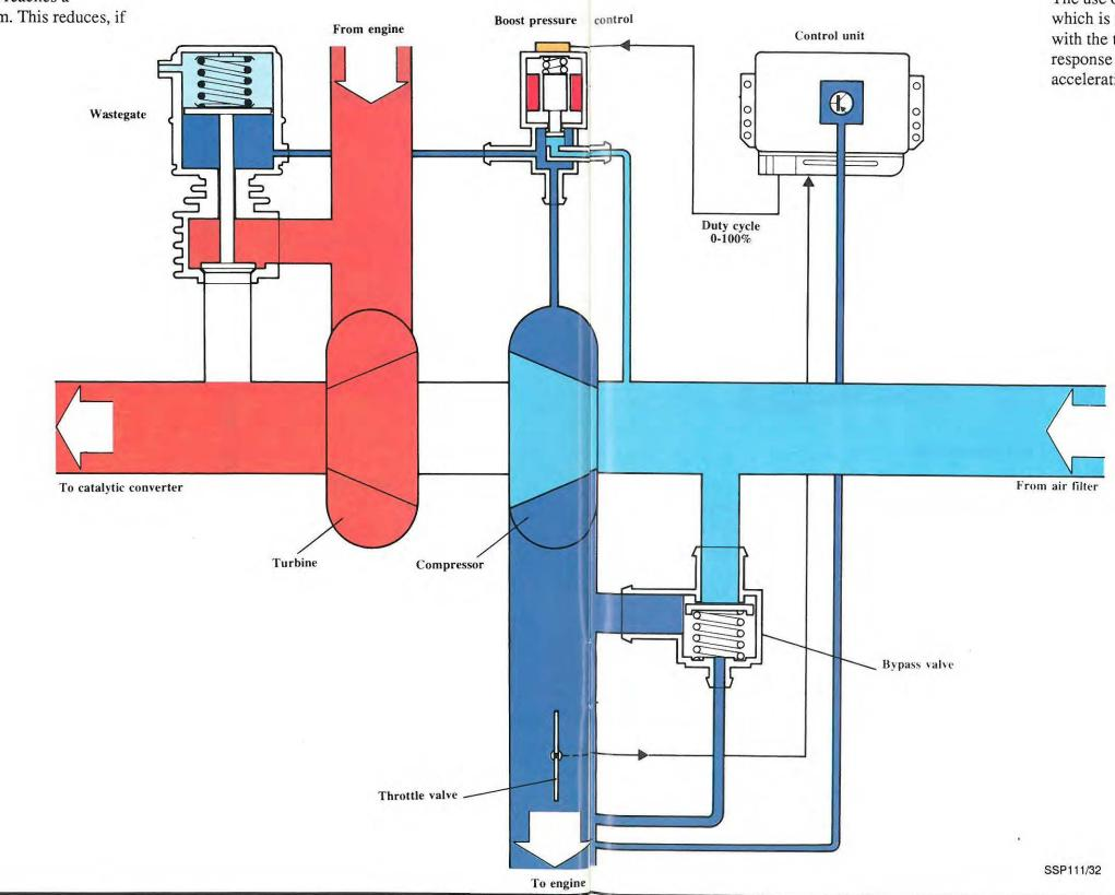
The bypass valve is used to reduce boost pressure in the intake air duct when the throttle plate is closed, such as, at idle or when decelerating.
