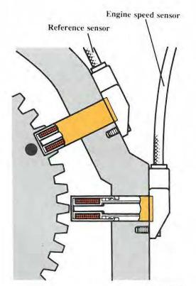
Both sensors are identical in design and are located on the left side of the engine compartment, near the flywheel.
