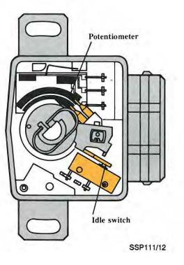
An idle switch and throttle valve potentiometer are used on the throttle assembly. The idle switch closes at approximately 1.3° before the throttle plate closes. When the switch is closed, this signal is used to activate the following functions:
