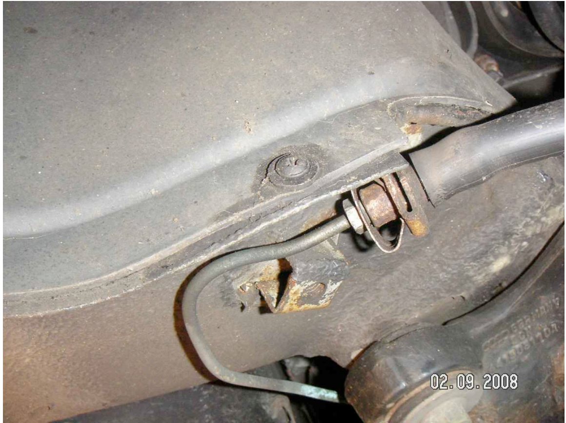
The Flare Nut (11mm) – where the steel and flexible brake lines meet. note: hanger and spring clip securing them to underbody of car
