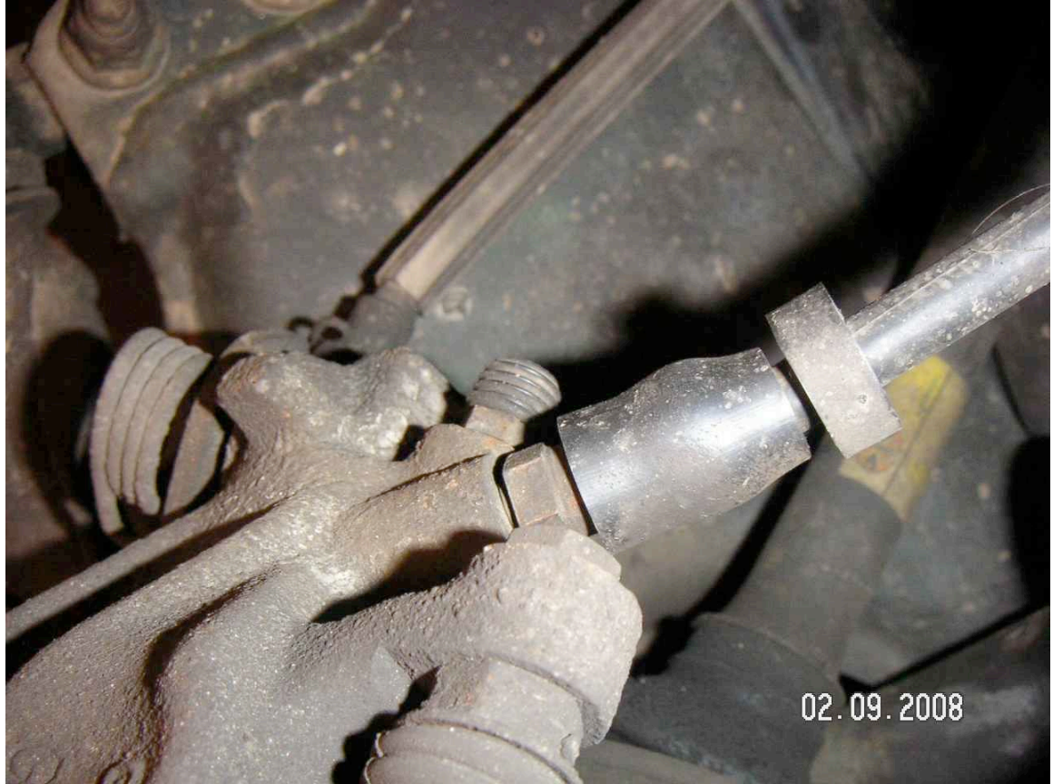
Flexible brake line where it screws into rear caliper (14mm wrench)
