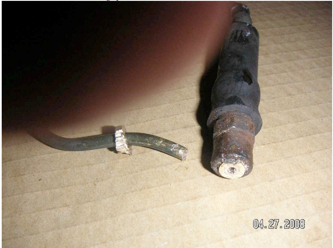
The old flare nut, cut by Sawzall
