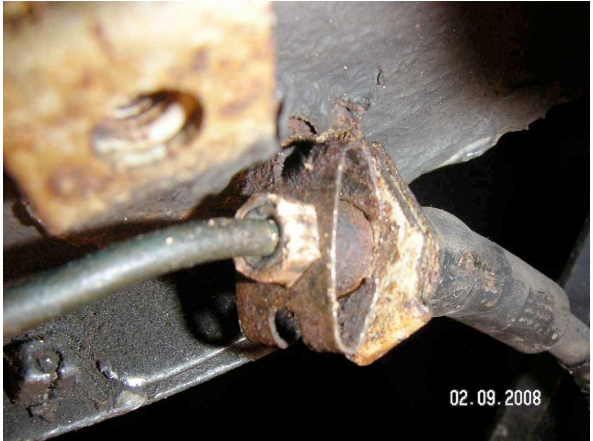
Ugly, ugly, ugly. Nothing's taking this nut off without a fight and likely a destroyed brake line.
