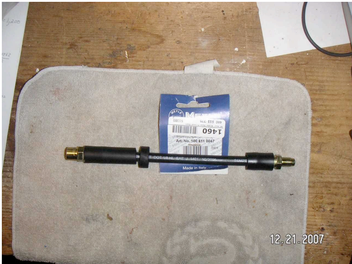
New Flexible Brake Lines. Caliper fitting at right, receptacle for Flare fitting at left.
