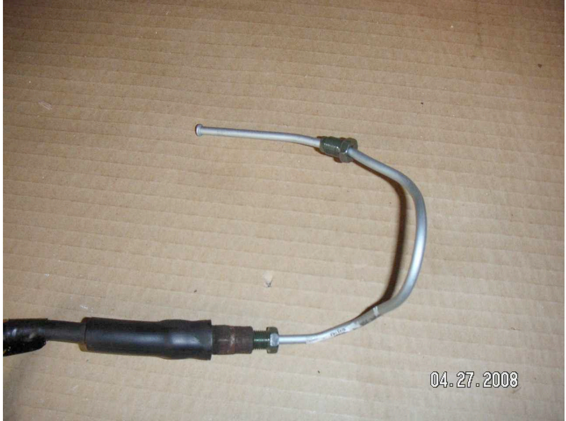
The new brake line, bent to fit. Expect to, ahem, practice ( aka, wreck stuff)
