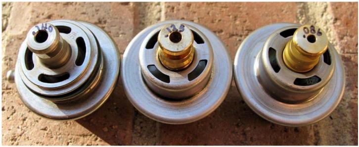
The work-around to get a better-suited C-series FPR is rather easy. It'll require 2 drill bits, ie; a number 36/.106" drill bit and an 1/8" (.125") drill bit and an electric/cordless drill
