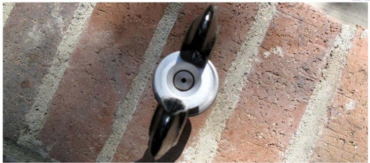
This shows the business end of the arrangement. I've purposely matched ID of the die to match the ID of the FPR housing where the small o-ring and outlet stem is held/sealed. This allows me to keep everything square and on-axis without it being such a fiddly affair
