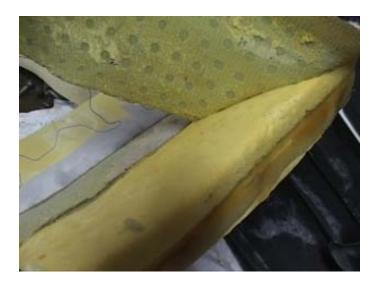
The new element is self adhesive. Working one section at a time, peel the backing and stick it to the cushion. Attempt to stick it in the same position that the original was. Route the wires through the slit or hole at the rear of the cushion.
