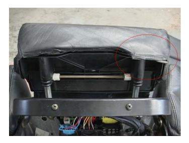
Now look at the rear of the base. Remove the two plastic sleeves from the posts where the torx bolts used to live. Loosen the 17 mm bolt that attaches the seat belt receptacle to the base and remove the plastic guard that is also attached to the torx bolt post. Slide the heavy cloth material and the leather off the post.
