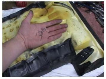
Peel the leather back and flip the cushion over again. Starting at the front, peel each section back to reveal a row of hog rings; there are three per row. Cut the rings to remove the leather cover.
