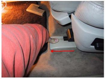
Remove the two mounting bolts (6 mm hex heads). Pull the front of the seat up, tilting it toward the rear to expose the wiring. Detach all the wires so that the seat can be removed. Make a mental note of the routing of the wires so you can get everything back together correctly.
