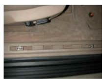
STEP 2: Remove the three Phillips screws that hold the door sill trim in place.
