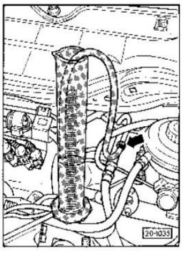
Attach hose to supply pipe and hold in measuring glass.
