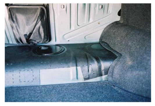
6. Remove the three screws in the cover plate and remove the cover plate:
