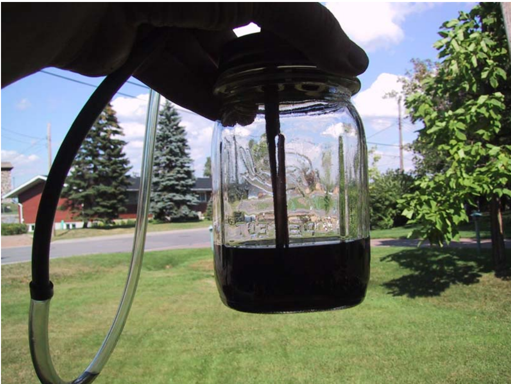
Photo 2 Old oil removed from bottom of reservoir
