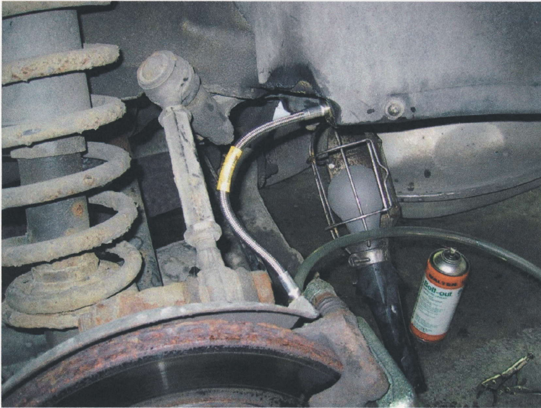
Photo 3 New SS Line Installed
