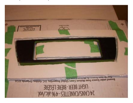
• Cover the surfaces of the lay-up surrounds will contact the carbon fibre and resin with wax paper cut to shape and taped to the lay-up surrounds. Make sure the wax paper lays flat and tight to the lay-up surrounds and does not bulge.
