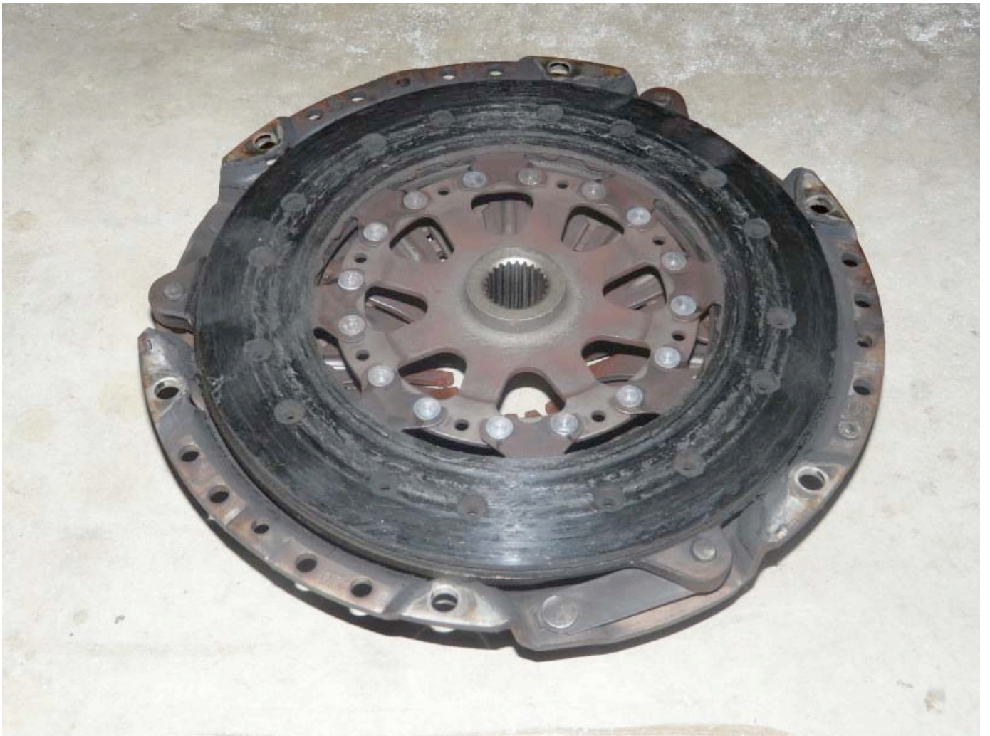
old oil soaked clutch removed.
