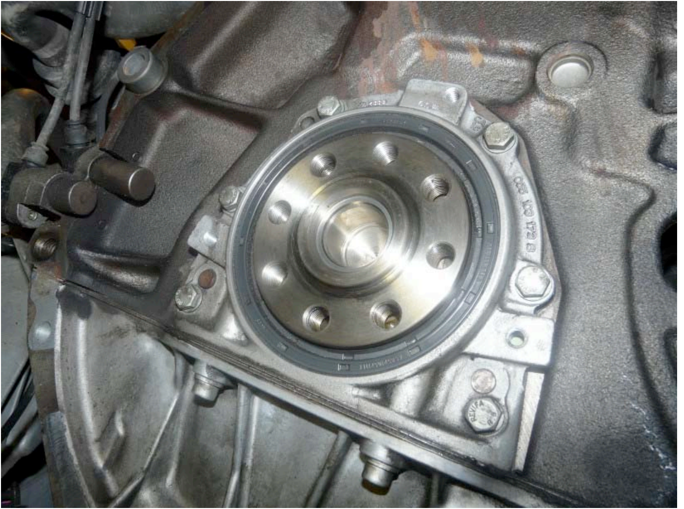
engine crank seal replaced
