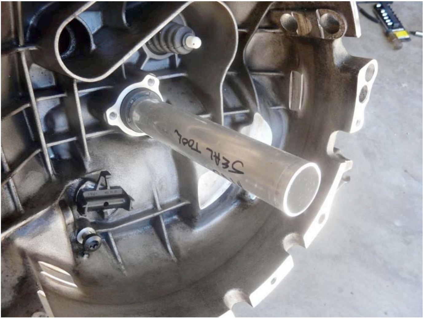
home made tool to drive in the tranny main shaft seal
