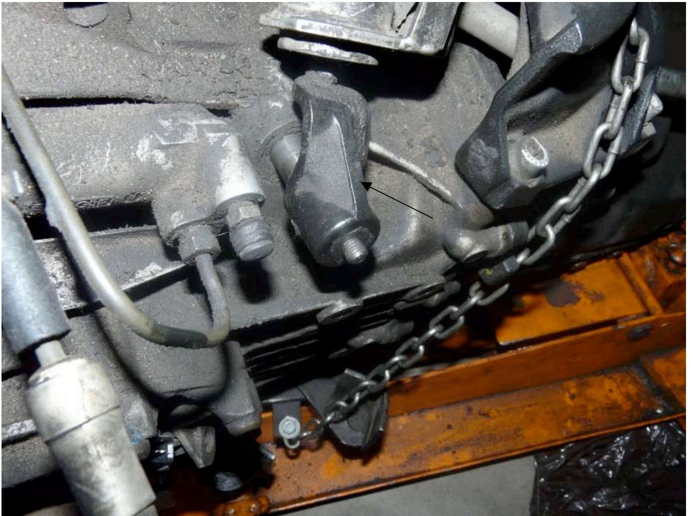
bell crank that needs to be removed from the shaft to get the shifter linkages to separate
