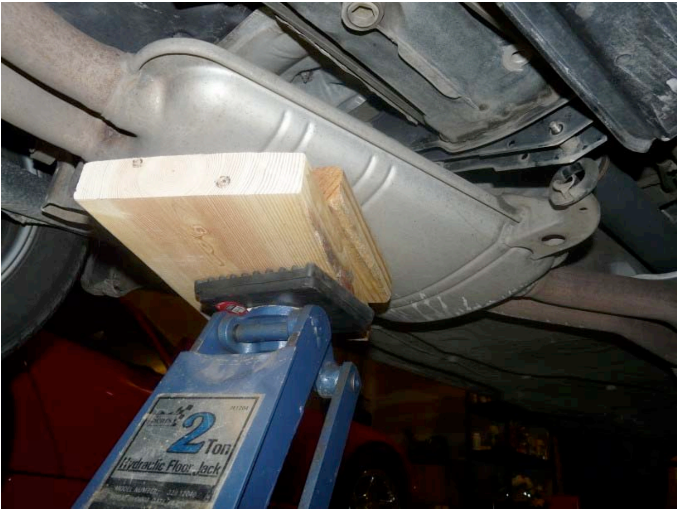
holding exhaust system while removing three flange bolts on each side, and removing rubber hangers This was fairly close to the balance point.
