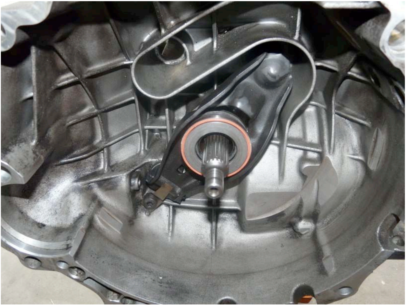
trans. ready to be reinstalled into car, with new throw out bearing
