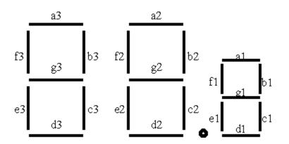
When a NO system electrical output is activated, a segment of the "88.8" display, indicated below as an alpha-numeric code, will illuminate. The decimal point in the "88.8" display will not illuminate in this channel.
