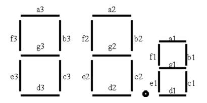
If an A/C compressor switch-off condition exists, a segment of the "88.8" display, indicated below as an alpha-numeric code, will illuminate.
