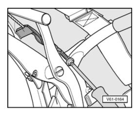
Fig. 2 Securing tensioning spring
