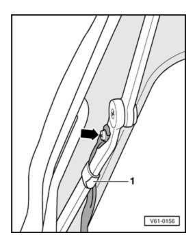
Remove adhesive tape - 1 - and remove retaining screws - **arrow** - for tensioning straps from frame linkage on both sides.
