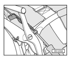
Remove screw for tensioning wire and pull tensioning wire out of convertible top cover from front.
