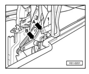
─Drill out rivet head - A - from linkage and remove tensioning strap - 1 - .
