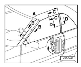
Adjust door window so that window glass is pressed against door seal over entire length of area - A - .
