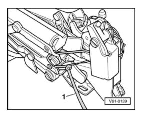
Fig. 1 Securing convertible top
