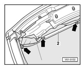
Remove screws - **arrows** - from retaining strip - **2** - on both sides.
