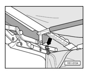
Remove headliner retaining screws - **arrow** - from convertible top frame on both sides.
