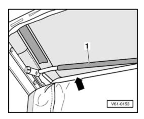
Clip headliner onto - 3 - cross rails - 1 - with 3 clamping strips - arrow - .
