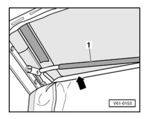
Disconnect clamping strip - arrow - from 3 cross rails - 1 - .
