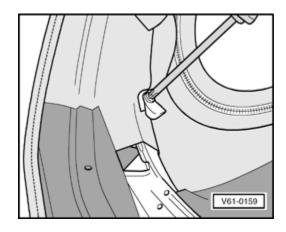
Remove Phillips-head screws from rear frame section on both sides and remove headliner.
