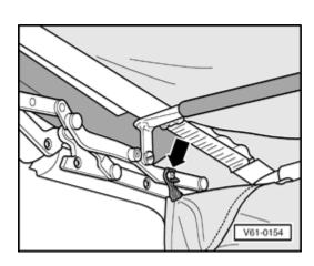
Remove headliner retaining screws - **arrow** - from convertible top frame on both sides.
