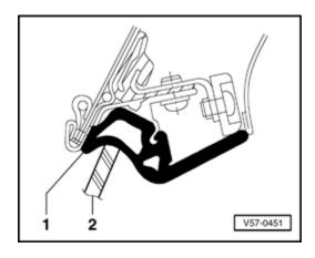
◆ Door window - 2 - must seal against door seal - 1 - as shown.
