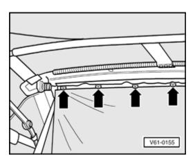
Remove screws - arrows - from rear cross rail and remove retaining strip with headliner.
