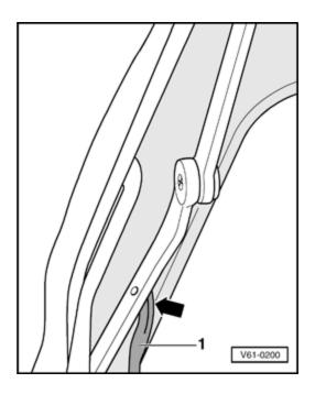
Secure tensioning straps - 1 - to convertible top frame linkage on both sides with screws - arrow - .
