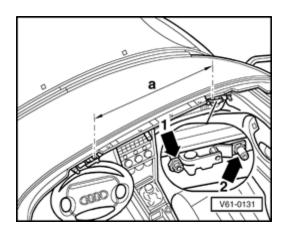
Fig. 1 Adjusting locking guide
