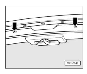
Remove screws - arrows - on front of front cover.
