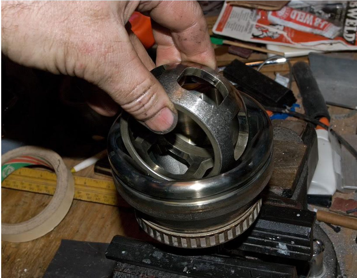
Notice wire tie on the ball cage, to keep track of 12 o'clock. I remark inner race and cage with Sharpie after a good cleaning.
