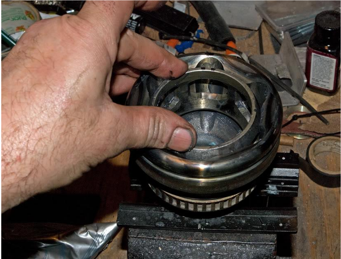
Grease coat and work inner race in at 90 degrees, fitting protrusions into ball cage slots until it's in a position to rotate freely.
