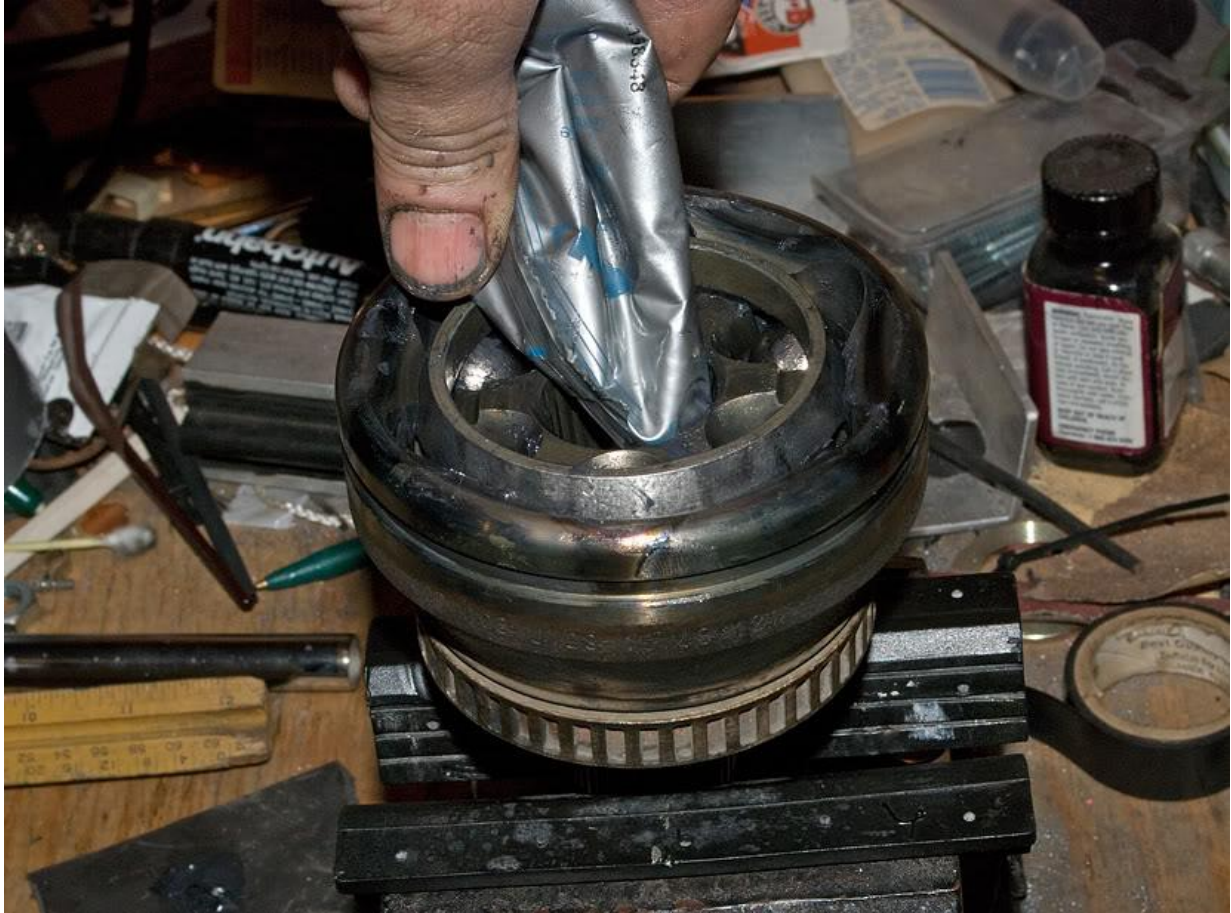
Packing tool: 19mm deep well socket with electrical tape sealing one end. I used my finger, but I like this method.
