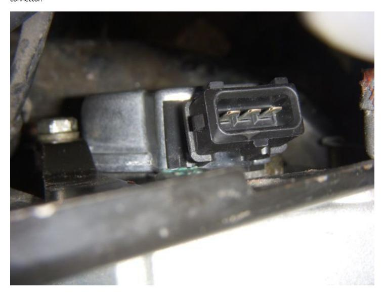
So the only things left to do was to put the connector on (push in the bail spring and push the connector on – it only goes on one way) and reconnecting anything else that you had disconnected (in my case the stupid cam cover ventilation tube).
