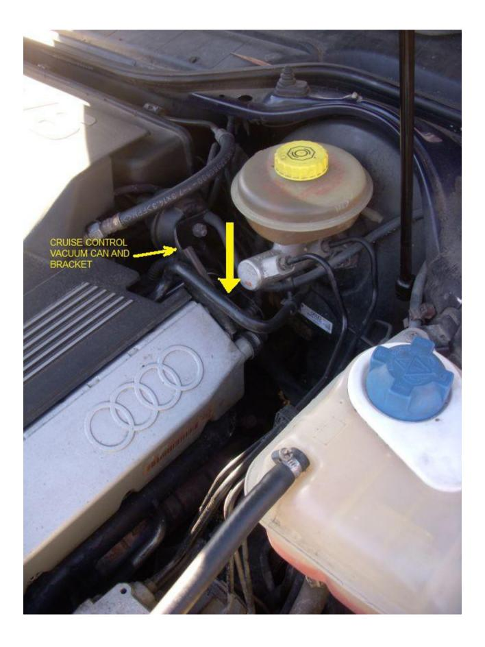
Here is a closer shot of the cam sensor connector and the cruise control vacuum can bracket (destined to cause a little grief) (Note: I HATE those pinch clamps that hold the vapour vent tubes to the cam cover):
