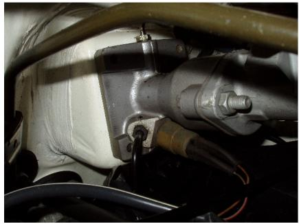
electrical leads to the brake servo. The two hydraulic lines visible above are the pressure line (lower next to the electrical connection) and the return line (on the top of the servo). These need to be disconnected. They take an 11mm flare wrench. I covered the ends with plastic caps and wrapped them in plastic while they were disconnected. It should be noted that one should not move the brake pedal with the lines removed from the servo.
