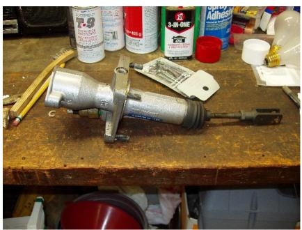
old servo and installed at the correct location on the new servo pushrod. I marked off the distance (230mm  $\pm$  0.5mm) on a piece of wood and placed it under the new servo with one end of the wood against the mating surface of the servo. After installing the locknut and the clevis on the new servo's pushrod, I
