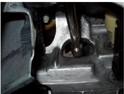
to rattle around the firewall for ever. For the blind nut, assemble the extensions one by one, feeding them through the small, rectangular hole in the brake support bracket as shown here. This is mostly a matter of feel. I could not see the nut no matter how I contorted, but others claim that they could – provided the extensions were ½ sized. When you have it, back it out gently. I lost this nut somewhere.
