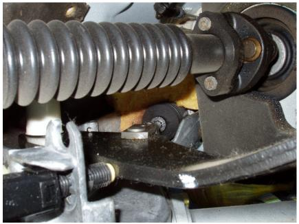
coming through the firewall and the clevis where it attaches to the brake pedal arm.
