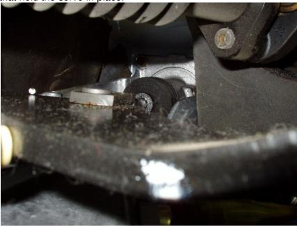
10. Visible in the above picture, you can just see one of the nuts after the sound insulation was removed. Three of the four nuts can be seen and accessed relatively easily. The fourth nut is blind and must be accessed by feel. Give your back a rest and move around to the engine bay.
