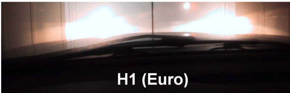
Photo 2 Beam Pattern H1 vs HID
