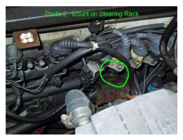
4. Note that the bolt comes up from the bottom of the bracket. It is secured by a metal tab bent over the bolt head (visible in the mirror in Photo 3). NOTE: THIS IS CRITICAL!!! If the bolt is not secured by the tab and the nut comes off, the bolt will drop down and jam on the transmission, locking the steering. THIS COULD RUIN YOUR ENTIRE DAY!
