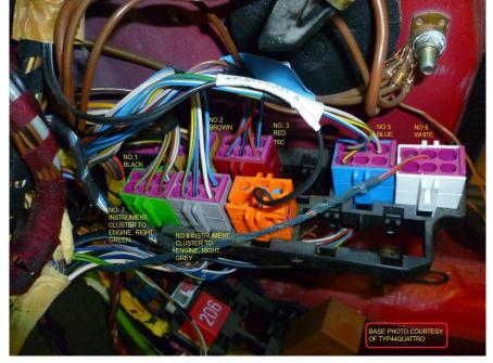
**1/6 Brown/Red** (0.5) Vehicle Speed Sensor (G22) (<u>More G22 Vehicle Speed Sensor info</u>) **3/6 Black/Blue** (1.5) from Fuse S14 in dash fuse panel, on to many devices, including back-up lights and ECU pin T55/22, via a <u>Data Link Connector</u> – as W/BL wire - linked to Check engine light (Malfunction indicator lamp) - also used in the <u>blink code check.</u>)
