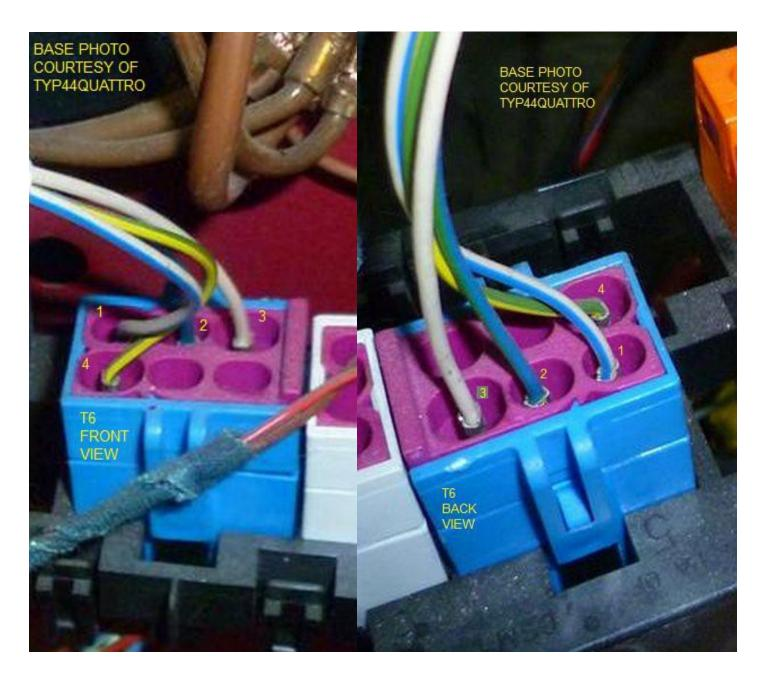
**Turbo Coolant pump relay (J155) (aka "324") has 5 connections. Blue 9 Pin relay plug.** For the <u>Auxiliary After-run Coolant Pump Relay</u> on the <u>Auxiliary Relay and Fuse Panel 3</u>
