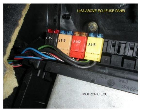
**Two wires with eyelet terminals**. One eyelet was removed from my loom but should be present on black wire. (NOT SURE ABOUT THIS ONE – INPUT APPRECIATED)
