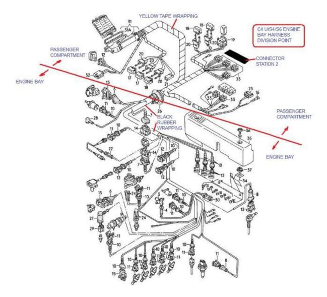
This current document is focussed on the portion of the harness that is wrapped in yellow tape and located in the passenger compartment, connected to Connector Station 1, Connector Station 2 and the instrument cluster (directly and indirectly):
