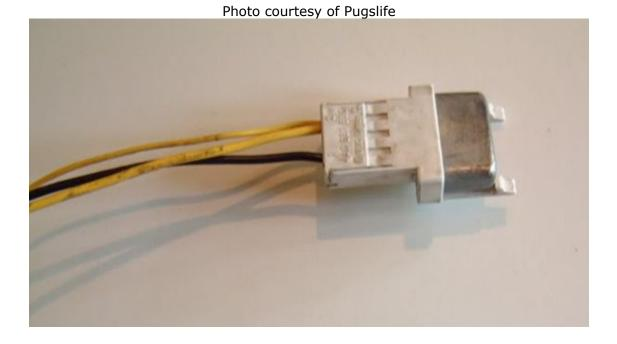
(S61 or S42?) Blue Fuse Holder (12Amp) on the Auxiliary Relay and Fuse Panel 3
