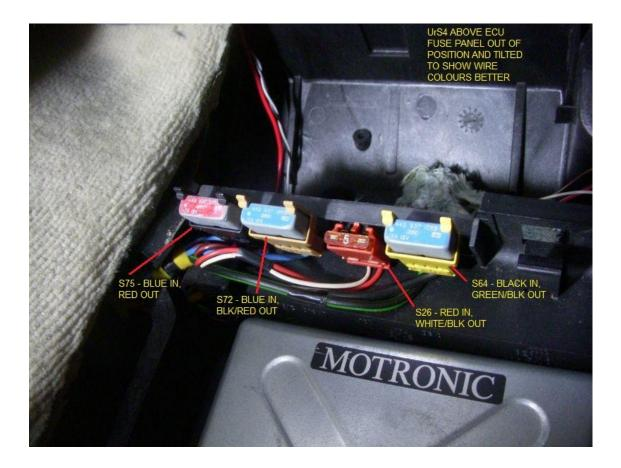
**Black Fuse Holder (12 Amp)** – S75 fuse for N71(ISV), N75 (WGFV) and N80 (Emissions canister valve). Stated as 10Amp ???
